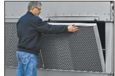
Framed Inlet Louver Design
