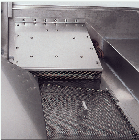
Bypass Connection with Diffuser Hood
