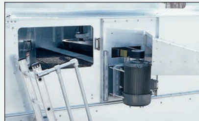
External Motor Mount (Optional Ladder Shown)
